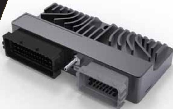
Spark advance calculation algorithms implemented in EMU BLACK allow high precision ignition timing up to 15,000 RPM and a wide range of supported trigger patterns. The trigger inputs are compatible with VR and Hall/Optical sensors (software selectable), with the ability to enable pullups / pulldowns, as well as analogue filters to fit any sensor configuration.
